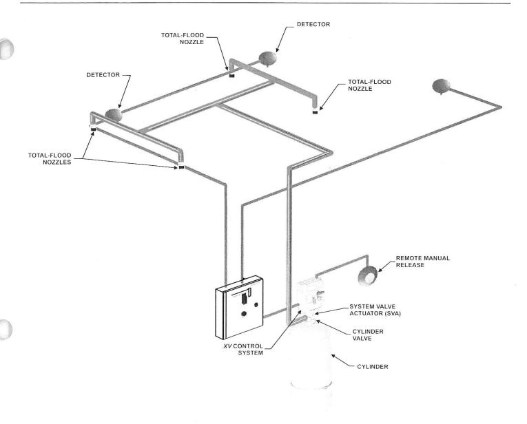
Figure 1-1. Typical Kidde<sup>®</sup> IND™ Dry Chemical System.
